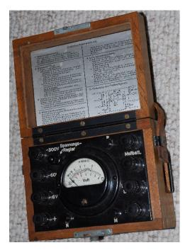
The feldmessgerät 30 can perform the following basic electrical test functions are supported; voltage testing, battery testing, resistance measurement and continuity testing. The operating instructions are written in German inside the cover. The feldmessgerät 30 can also self test,
